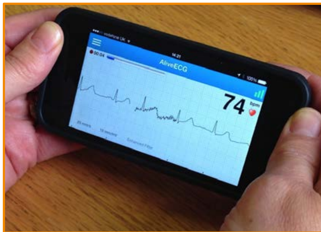
Figure 5: an example of AliveECG, a portable ECG that allows to check one's heart rhythm.
